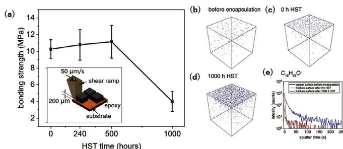
Fig. 1 (a) The bonding strength results for different lead frames under various reliability tests. (b) 3D render images of epoxy fragment  $C_{15}H_{26}O-$  for the copper surface before encapsulation and the fracture surface of the copper substrate after (c) 0 and (d) 1000 h HST; (e) depth profile of  $C_{15}H_{26}O-$  for the copper surface before encapsulation and the fracture surface of the copper substrate after 0 and 1000 h HST.
