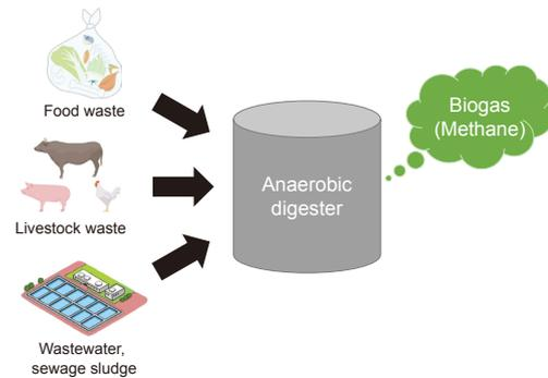
Biogas (methane) production from organic waste/wastewater by anaerobic digestion
