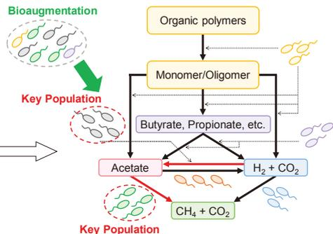
Ammonium/salinity inhibition of metabolic pathways in anaerobic digestion and its mitigation through bioaugmentation with tolerant microbial community
