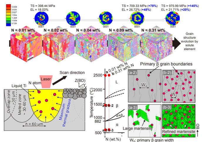
Figure 2. The transformation of grain structure resulting from an increase in N concentration, elucidating through the utilization of 3D IPF mappings for  $\alpha$ -Ti, complemented by schematic representations that depict the microstructural changes occurring during the rapid solidification process.
