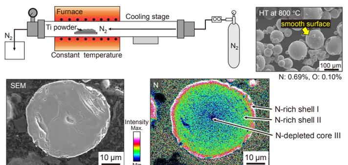
Figure 1. The modification of Ti powder via gas-solid interactions process at an elevated temperature presents a method that affords two noteworthy advantages. Firstly, it maintains the exceptional flowability of the feedstock. Secondly, it ensures the potential for the even distribution of N following the fabrication process.
