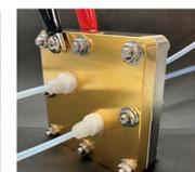
Membrane electrode assembly cells
