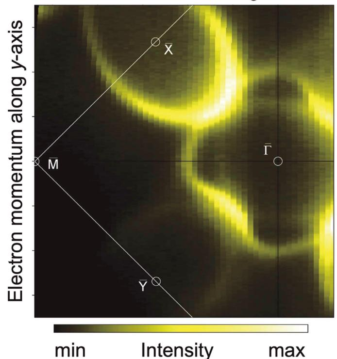
Fig. 2 The Fermi surface of the surface electronic state obtained with an angle-resolved photoelectron spectroscopy. The intensity is extended in a diagonal direction, which does not reflect to the four-fold symmetry of bulk crystal structure but to the two-fold symmetry of the surface structure.
