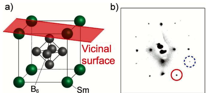
Fig. 1 a) Crystal structure of samarium hexaboride ( $\text{SmB}_6$ ) and the vicinal surface. b) The electron diffraction pattern of the vicinal surface. The intensity difference between spots marked by solid and dashed lines reflects the anisotropy.
