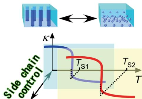
Fig 1 Tuning the switching temperature in thermal switch using the order-order transition in liquid crystalline block copolymer. Choosing the type of mesogens in the side chain in liquid crystal part modulates the switching temperature.
