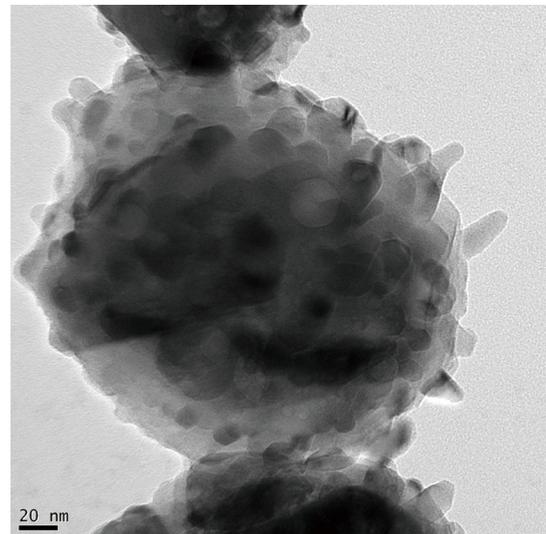
Ceramic particles covered by nickel oxide
