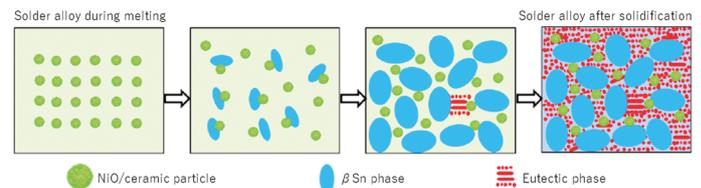
Solidification microstructure of solder alloy with ceramic particles covered by nickel oxide
