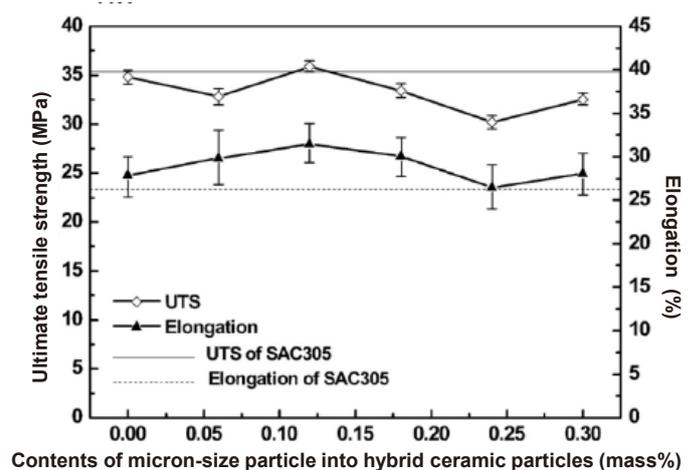
Mechanical properties of composite solder alloys reinforced with hybrid ceramic particles
