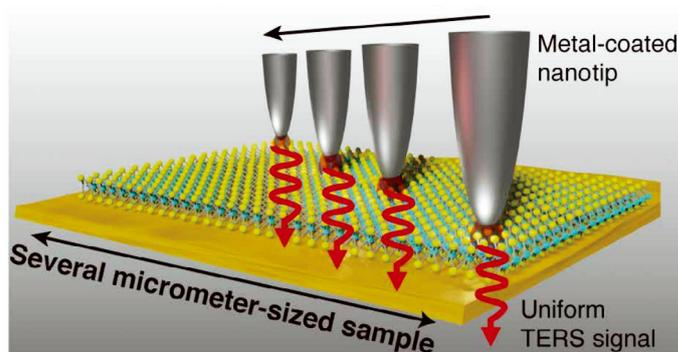
Overview of ultrastable near-field Raman Spectroscopy
