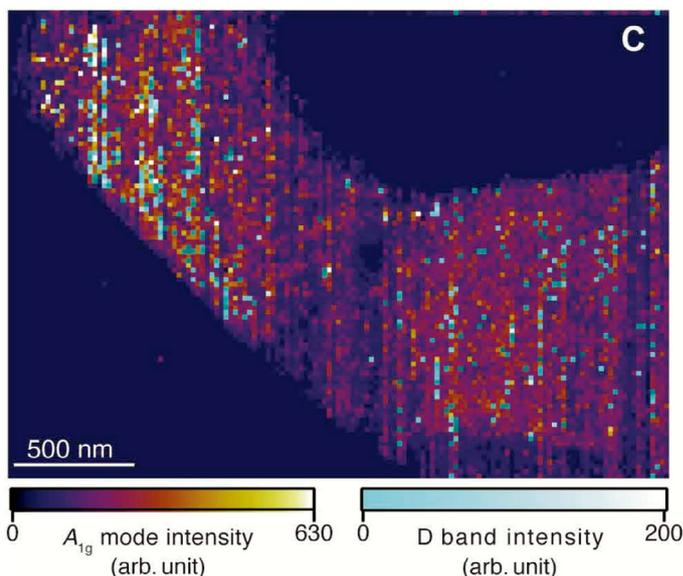
Large-area super-resolution Raman image obtained of MoS<sub>2</sub> through 6-hour imaging
