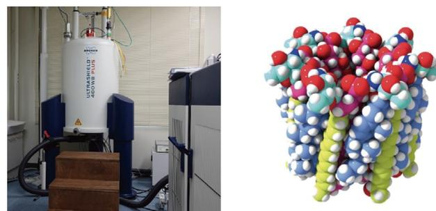
Figure 2. 3D molecular configuration information was obtained using a solid-state NMR system (left), and the structure was assembled to satisfy these requirements (right).
