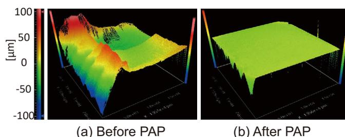
Fig. 1 Flatness of single crystal diamond substrate
