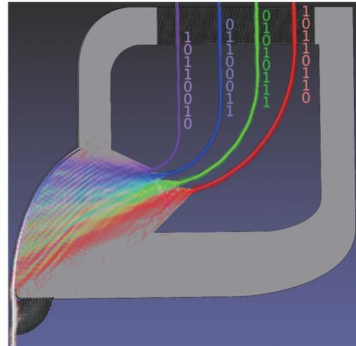
Schematic of the integrated multiplexer, showing broadband terahertz wave being split into four different frequencies, where each is capable of carrying digital information.
