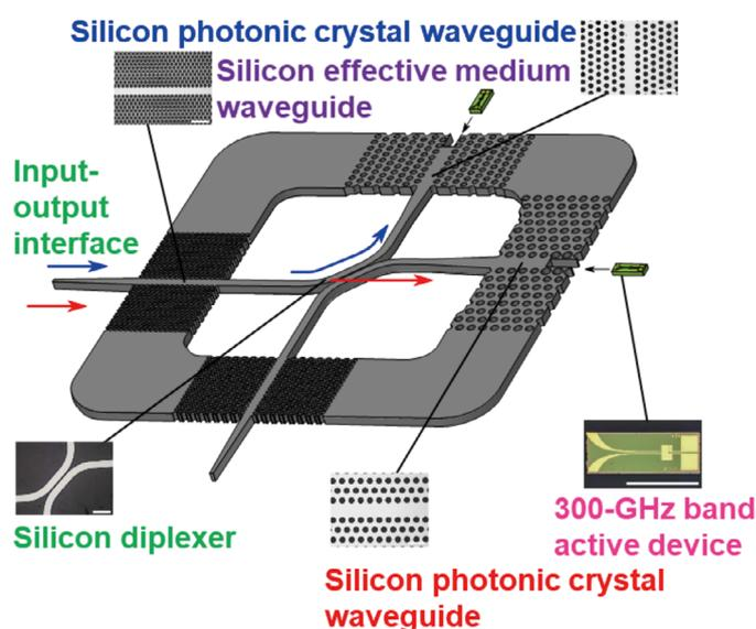
Developed terahertz circuit based on terahertz silicon photonics
