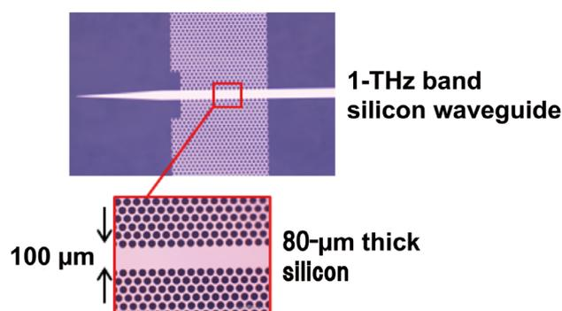
Fabricated one-terahertz band silicon waveguide
