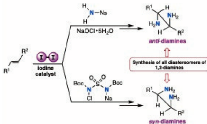
Fig. 1 Stereospecific 1,2-Diamination Enabled by I 2 Catalysis
